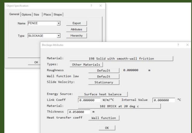
For a non-participating BLOCKAGE (material 198), it is possible to set a heat balance boundary condition for the surface temperature.
