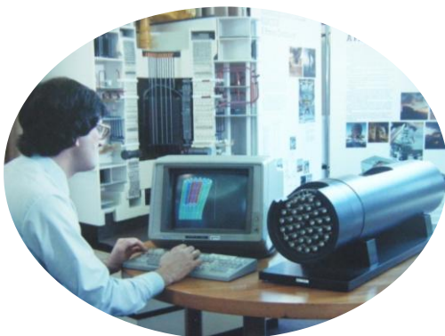
Figure 1. A young Dr Robert Hornby displaying a damaged fuel pin bundle on a Tektronix graphics terminal. A model of the British AGR is shown in the background. To the right of the display terminal is a model of a full size (undamaged) AGR fuel element incorporating 36 fuel pins in a graphite sleeve.
