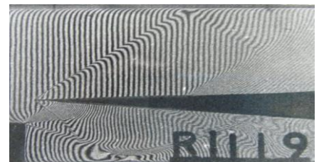
Figure 2. Interferogram of the steady two dimensional flow of nitrous oxide at M_f=1.56 past a wedge whose upper surface is inclined at 2^\circ to the freestream, showing broadening of the wave (due to vibrational relaxation) away from the upper wedge surface.
