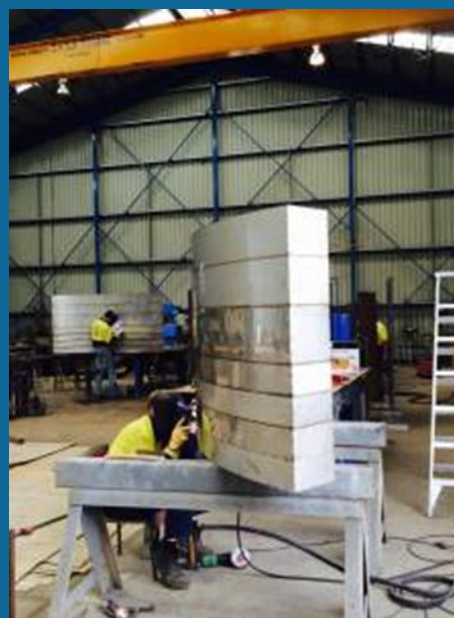
Figure 2. An array of MTSWDs being prepared for use in the Brighton Tower. Note the different box depths.
